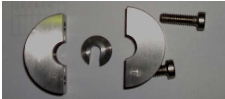
Figure 5-10 Noodle Flexure Clamp assembly stamped "H"
