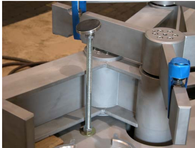
Figure 4-25 screw jack, with the swivel foot, padded with neoprene rubber
