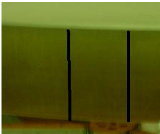
Figure 4-11 temporary fiducial marks on the side of the mirror
