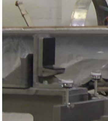
Figure 4-3 Seismic Restraint with SR Bracket 3 removed
