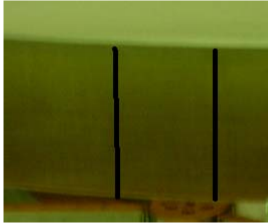
Figure 4-27 temporary marks to show indexing of mirror or placement of lifting device
