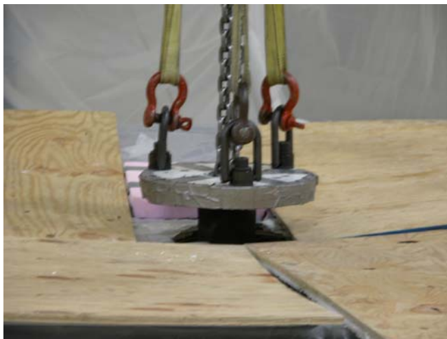
Figure 4-1 Example of lifting device shown with tissue, foam and plywood for protecting mirror
