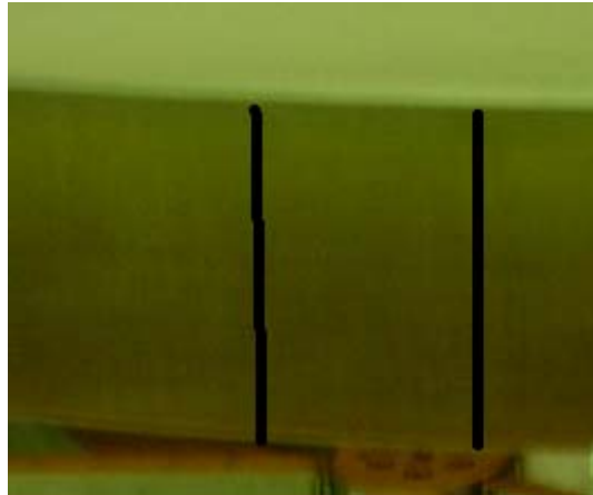
Figure 5-1 temporary fiducial marked on edge of mirror to mark a lifting device or Seismic Restraint location
