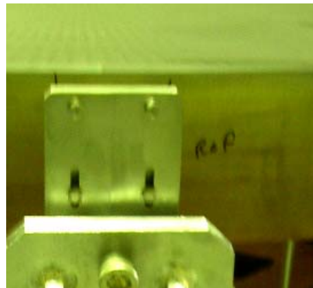
Figure 5-2 temporary fiducial aligned with Seismic Restraint
