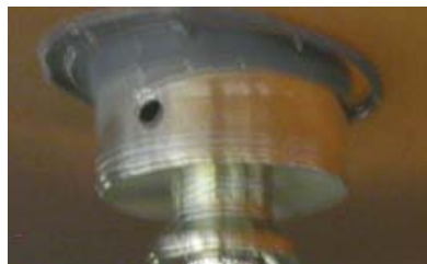
Figure 4-14 axial Invar Puck permanently bonded to mirror
