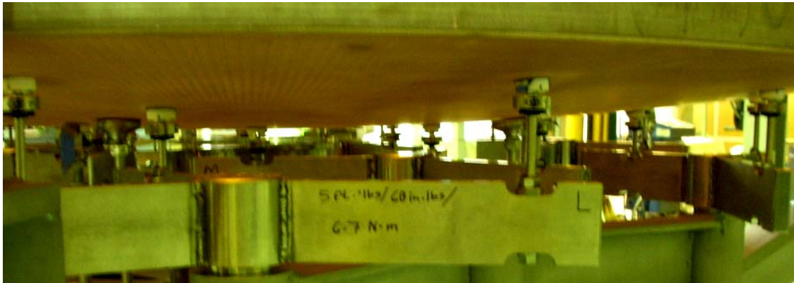
Figure 4-7 location of a Noodle Flexure Clamp assembly labeled “L”
