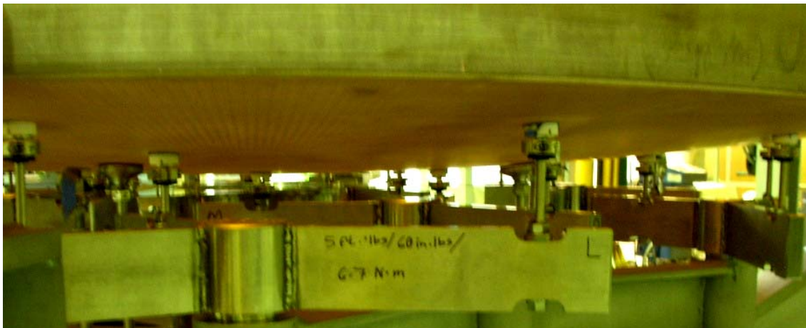
Figure 5-11 location of Noodle Flexure Clamp assembly marked "L" on Support
