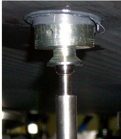
Figure 4-23 shows 1 of 27 axial Invar Pucks mechanically disconnected from Noodle Flexure Assembly by removal of Noodle Flexure Clamp assembly
