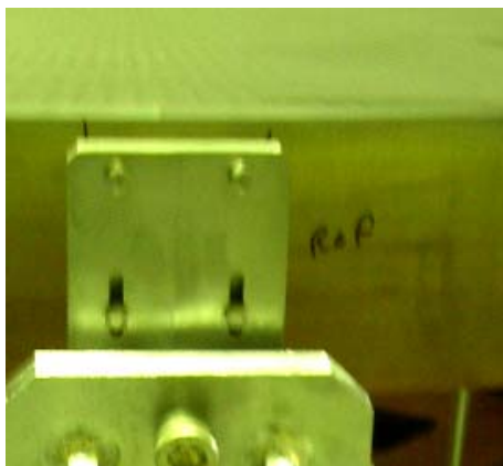
Figure 4-12 notice temporary fiducial marks above Seismic Restraint on side of mirror
