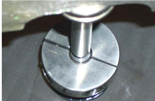
Figure 5-14 gap on Flexure Clamp assembly is nearly symmetrical and in an acceptable condition
