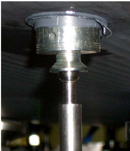
Figure 5-8 sphere of axial Noodle Flexure Assembly engaged into cone of axial Invar Puck, 1 of 27 places
