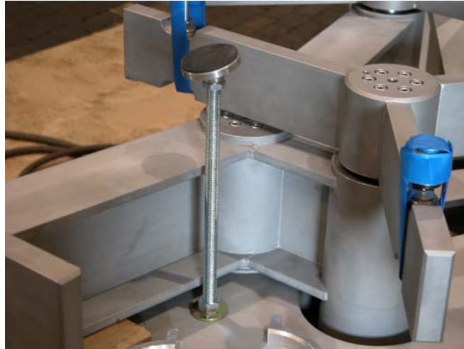
Figure 4-16 jacking screw with the swivel feet padded with neoprene rubber
