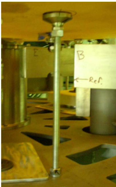
Figure 5-7 mirror lowered onto screw jack
