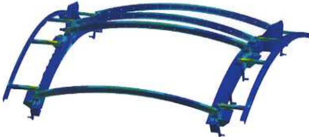
Figure 5.6.: Shutter Survival Condition – Von Mises Stress
