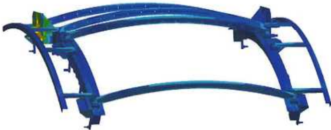
Figure 5.7.: Shutter Operating on one chain – Von Mises Stress
