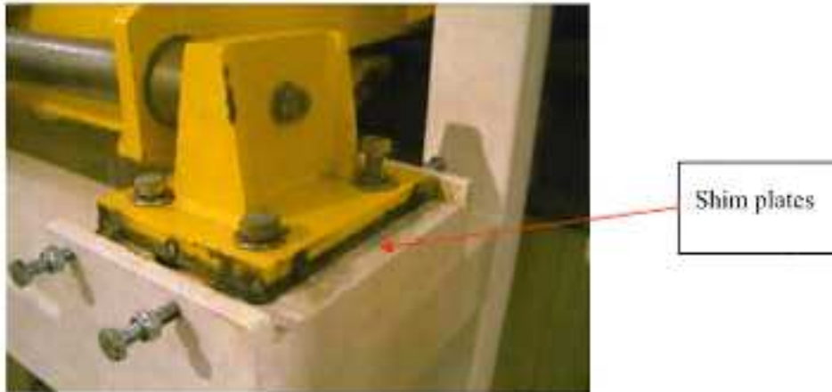
Figure 18 Azimuth drive assembly shimming
