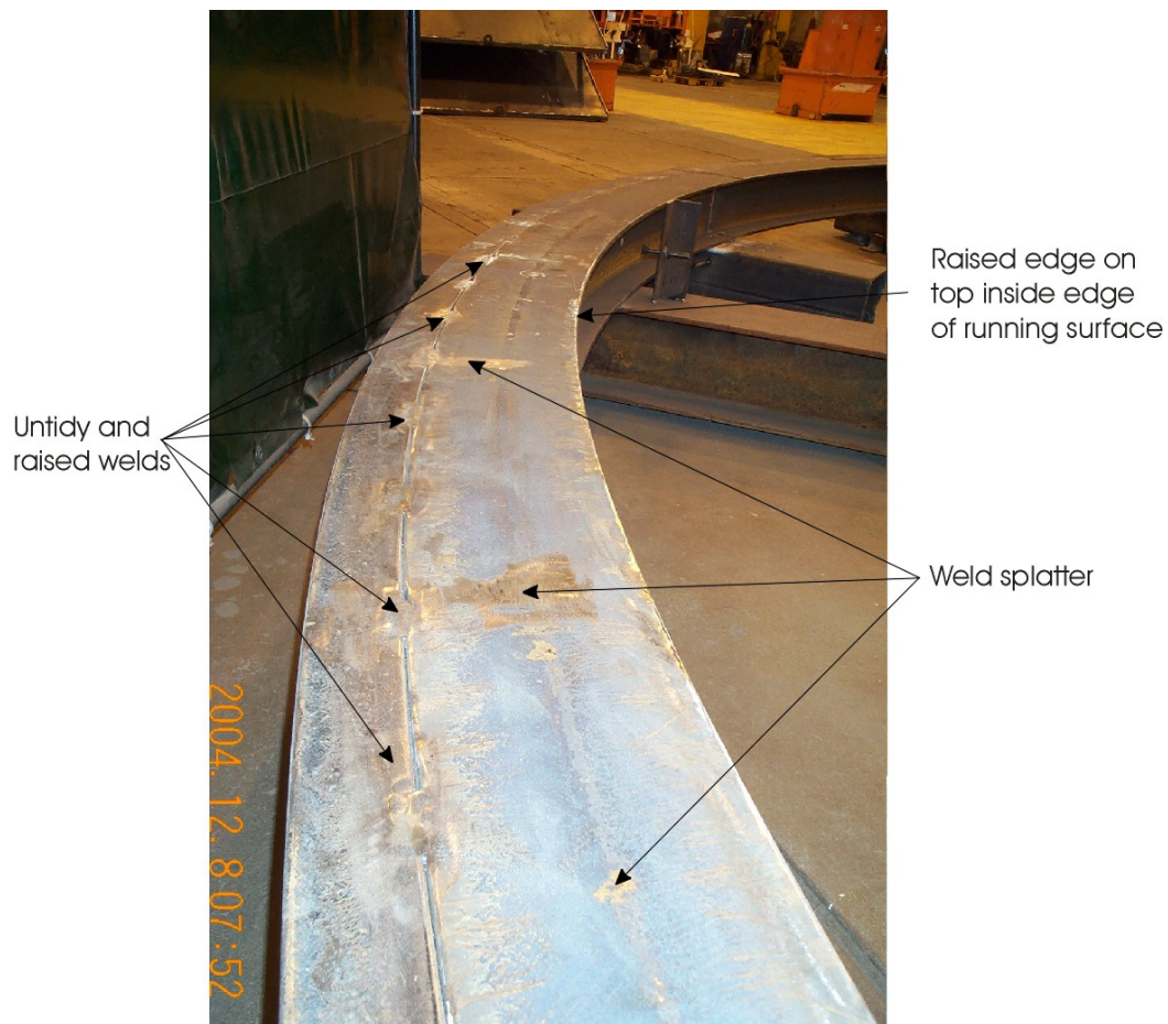
Figure 2-1 Ring beam RI issues addressed
