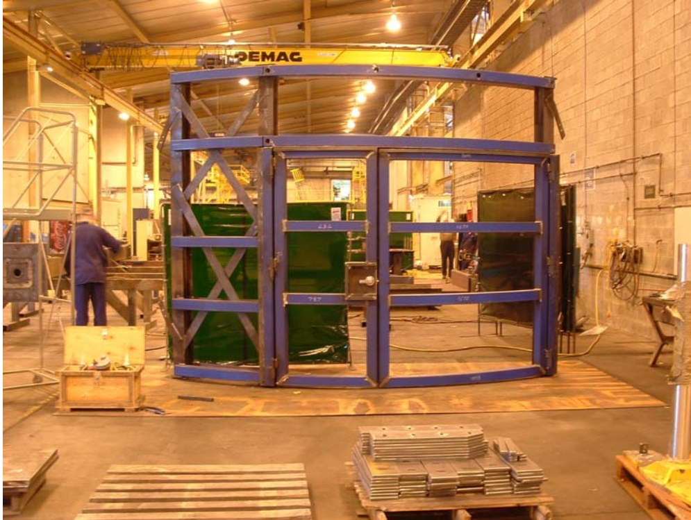
Figure 2-5 Ring wall equipment door
