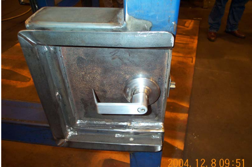
Figure 2-10 Untidy welds on door lock housing plate
