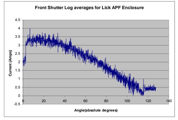
**Comments:** Reference is the arch beam spring line. Marker was the front shutter mid point. Travel was from front of the enclosure to the rear (negative travel direction.)
