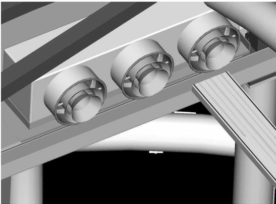
**Figure 5. Level 4 Fan Coil: Enclosure Cooling**
