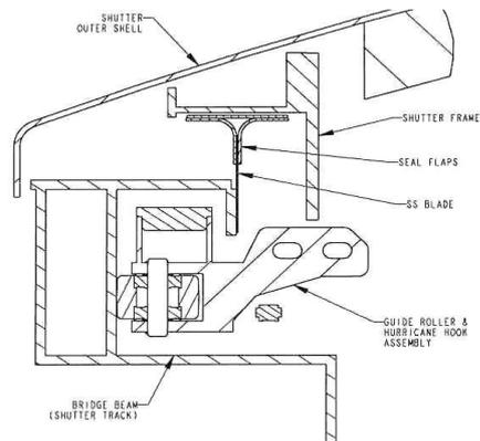
Figure 8. Series I Shutter Longitudinal Seal
