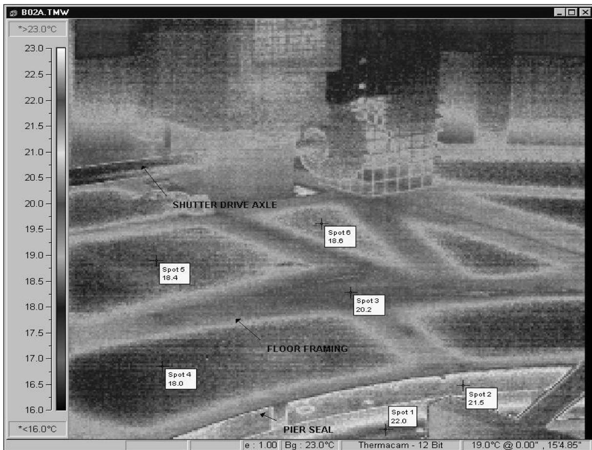
**Figure 13. Thermograph B02A (Level 2 Floor and Pier Seal)**
