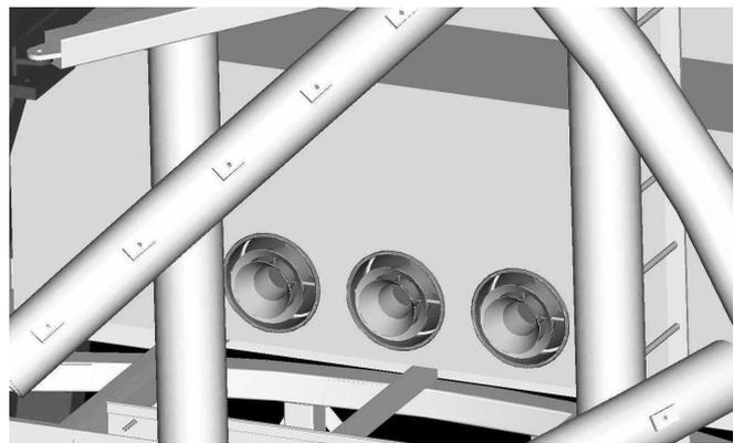
**Figure 6. Level 2 Fan Coil and Jet Diffusers: Mirror Cooling**
