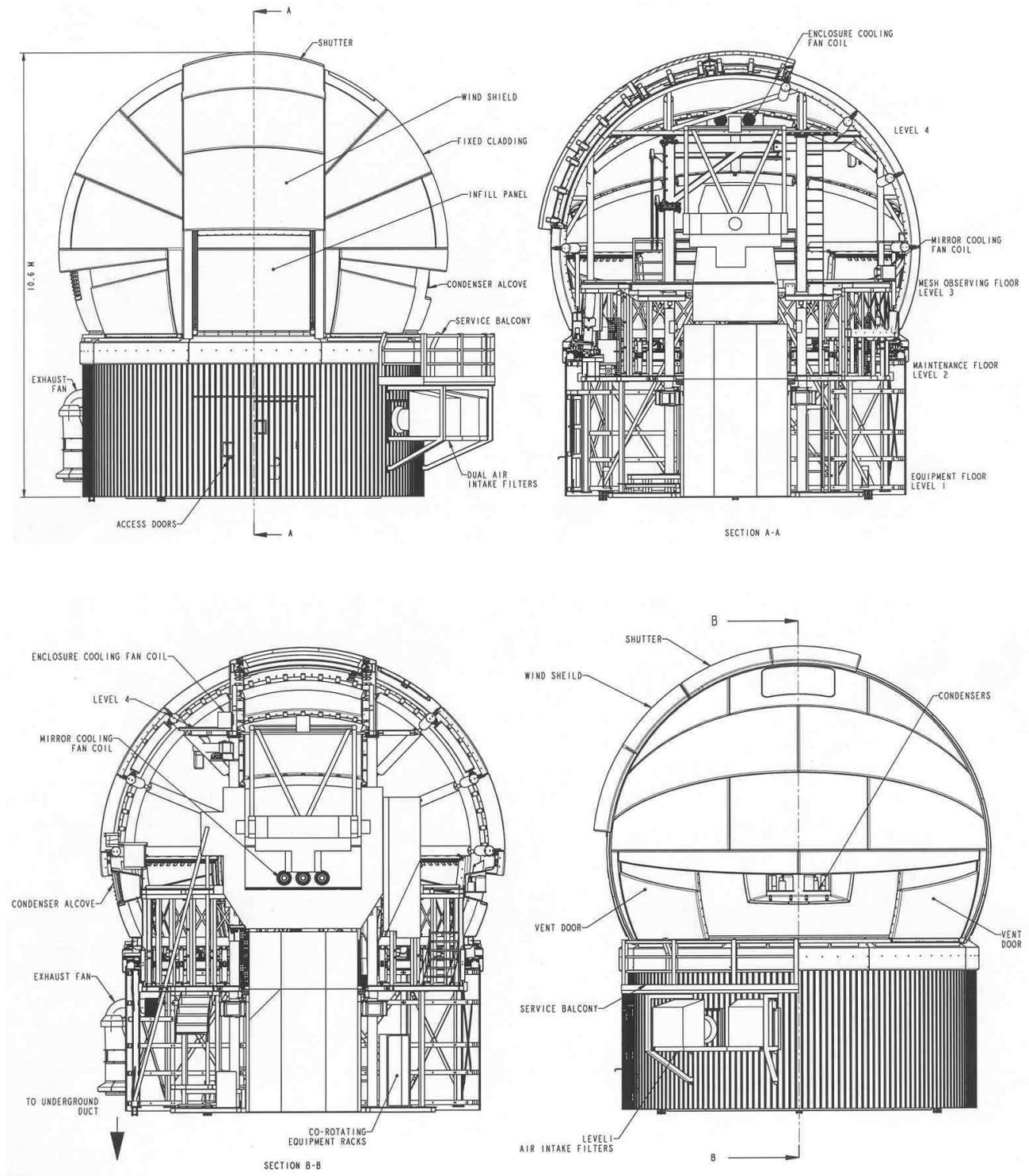
**Figure 4. Section Views of the IceStorm Series I Enclosure**
