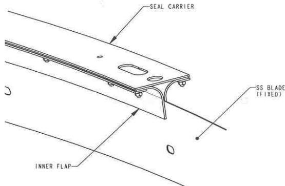
Figure 7. Azimuth Dual Flap Seal
