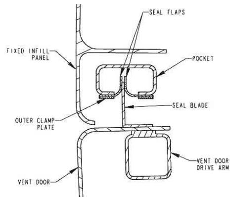
Figure 9. Vent Door Pocket Seal
